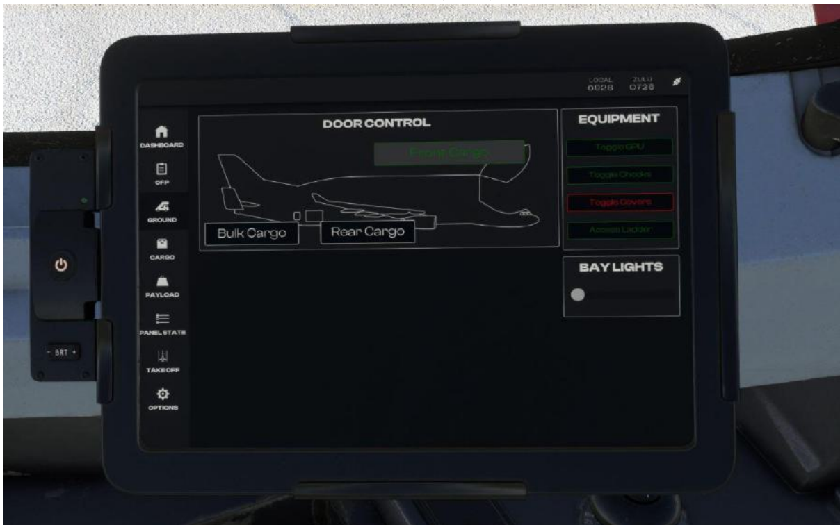
Ground Page – Controls doors on the aircraft along with requesting external Ground Power, chocks, covers and illumination of the cargo bay.
