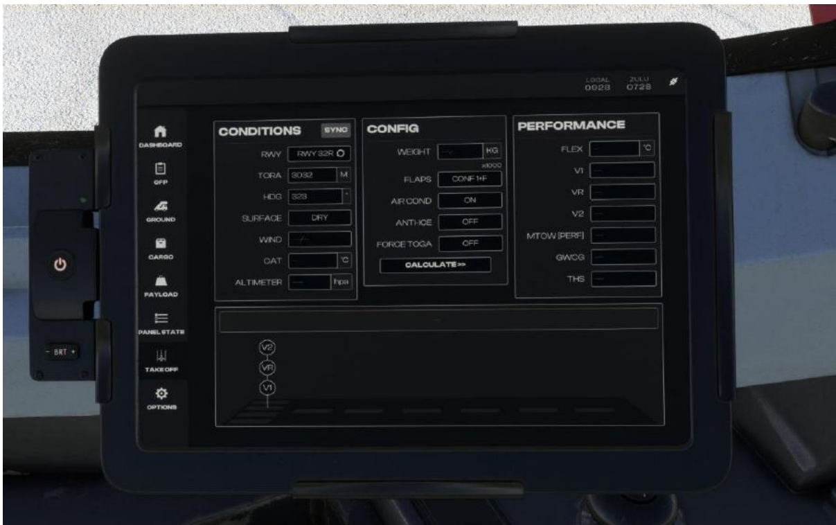
Takeoff Page – This page allows you to set the conditions for takeoff to calculate your performance references.
